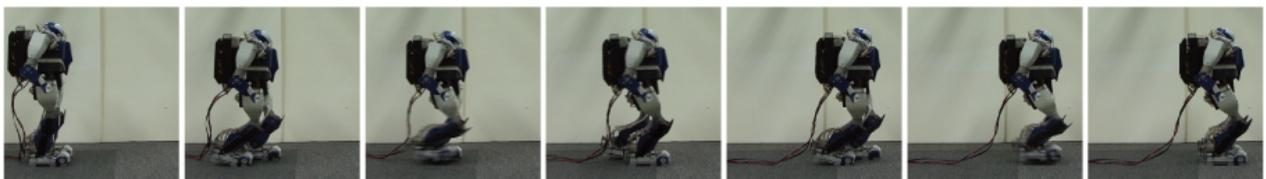
Fig. 2 Snapshots of the walking motion including toe support phase
