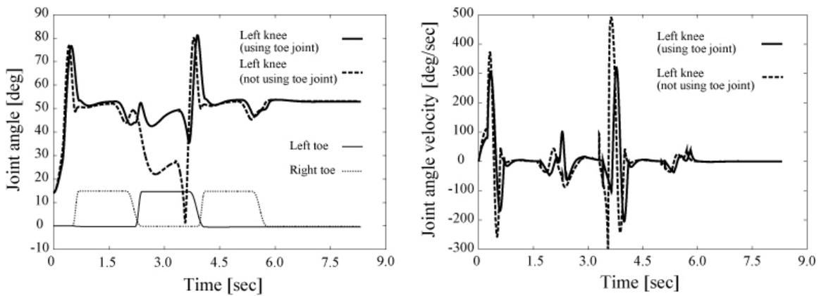
Fig. 4 Loci of the knee and toe joint angles, and the knee joint angle velocities
