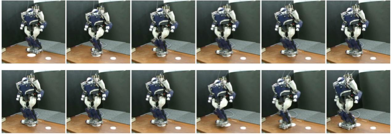
Fig. 5 Snapshots of walking experiment on the ground with a plastic plate. Applying impedance control, the robot carried out the total four steps walking motion.
