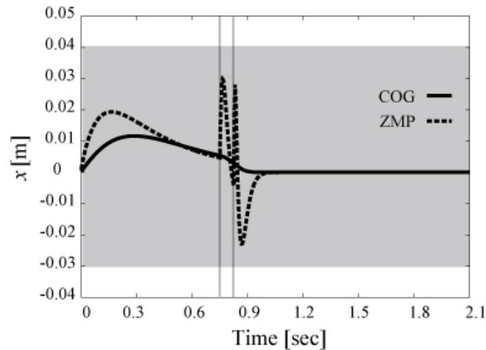
Fig. 7 Initial response of the system when switching control applied. At 0.75[sec] and 0.84[sec], controller switched the compensator.
