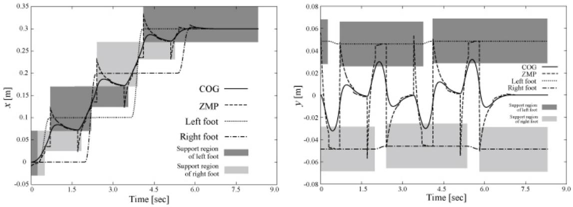
Fig. 3 Planned COG and ZMP for walking motion including toe support phase
