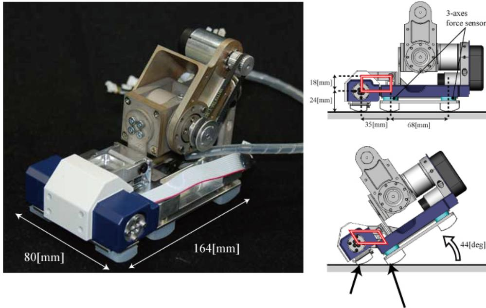
Fig. 1 Toe-Thenar mechanism with parallel four-bar linkage
