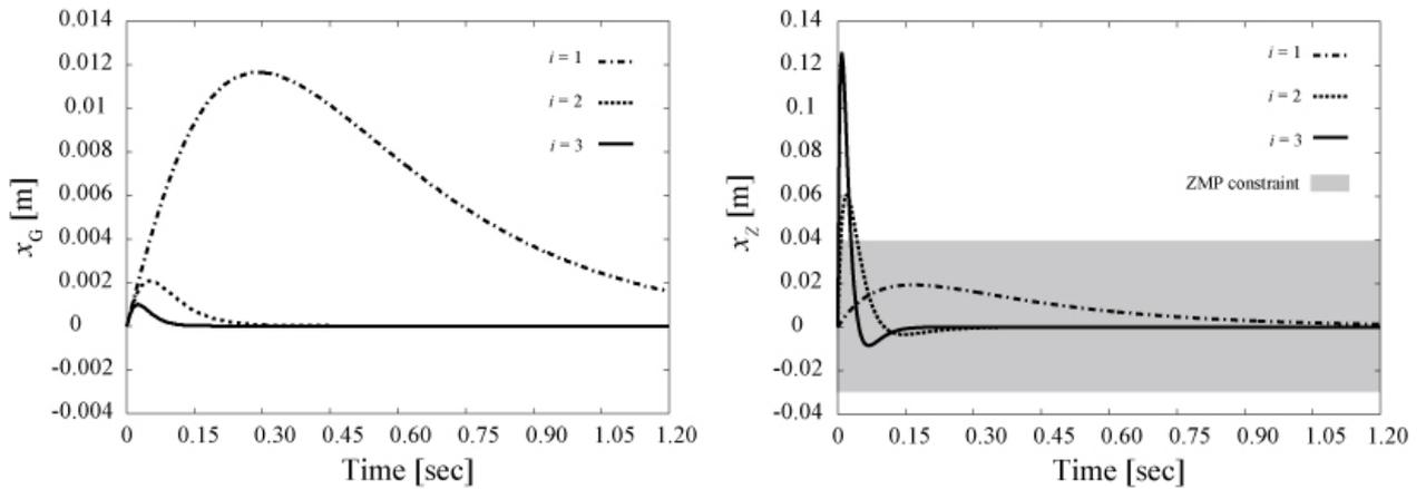
Fig. 6 Initial response of the system. The left and right are response of COG and ZMP, respectively.
